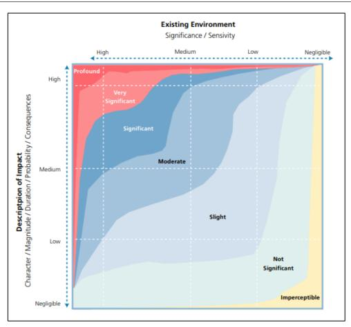
Figure 13.2: EPA Chart Showing Typical Classifications of the Significance of Effects<sup>3</sup>
